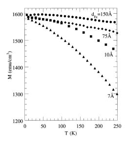
Fig. 1. Magnetization versus temperature for  $d_{Fe} = 150$  Å (circles), 75 Å (diamonds), 10 Å (squares) and 7 Å (triangles) samples.
