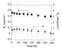
Fig. 4. Interface (squares) and bulk (diamonds) anisotropies as a function of temperature.
