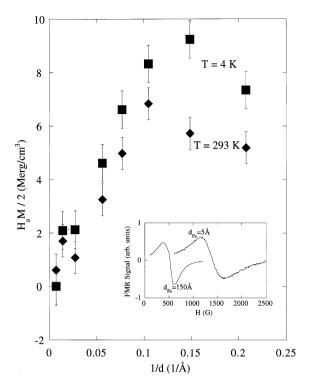
Fig. 3. Intrinsic anisotropy energy as a function of inverse Fe layer thickness. (See model in text.) Error bars are estimates obtained from uncertainties in magnetization and resonance position. Note deviation from linearity for the thinnest samples.
